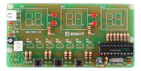
Step 15:Install 1pcs TO-92 78L05 Voltage Regulator at U2.
